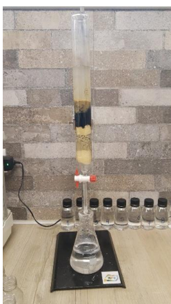
Figure 5 - Laboratory filtration with Activated Carbon and Diatom Stones
