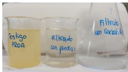
Figure 13: Comparison of filter with stones and activated carbon
