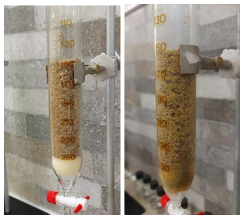
Figure 11 – Resins before and after adsorption
