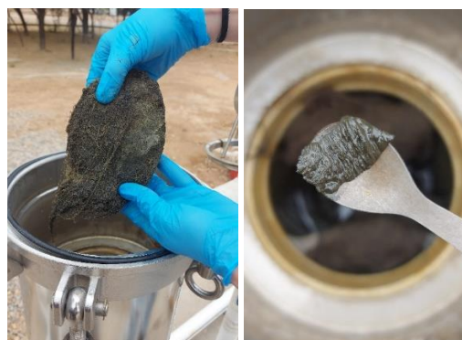
Figure 12 - Filter after 26 hours of operation
