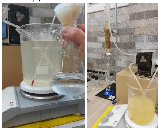
Figure 9 – Hot filtered brine before entering columns and cold filtered brine
